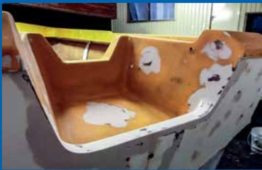
advance his new project from bare hull to a fully-refurbished runabout. The process started with the gruelling task of grinding and filling fibreglass, sanding and masking.
