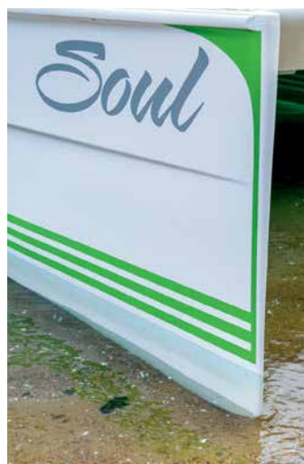
ABOVE Retractable fins keep the cat tracking straight when running on one engine.
